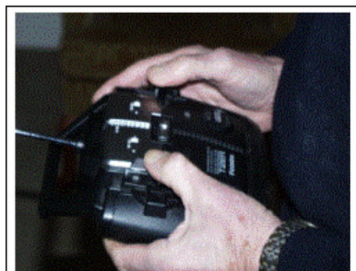
Transmitter held in hands and operated with thumbs. Note short sticks
