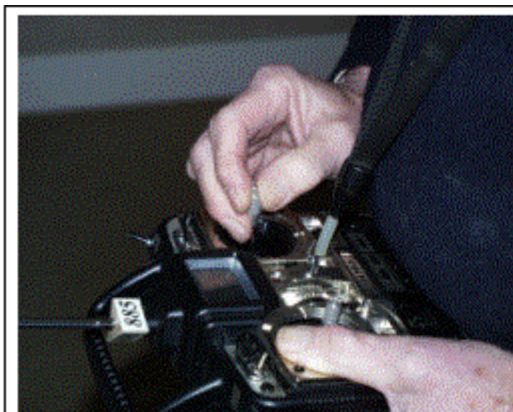
Single stick operation using penholder grip Transmitter suspended from neck strap and stabilized with left hand. Note long stick
