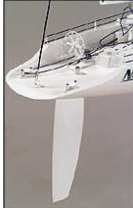
Above: the large high aspect ratio rudder is very responsive.
