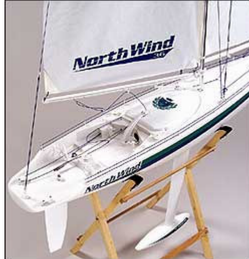
A nice, wooden stand comes with the kit. Note the exposed rudder pushrod. Adjustments to the clevis are easy.
